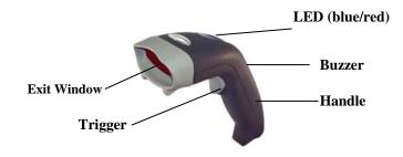
When a barcode is successful decoded, the blue LED light of the scanner will turn on and off. The scanner will beep once. If the barcode is not successful read, the LED will show red and the buzzer will not sound.
