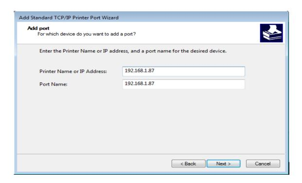
Enter the IP address of the printer Ethernet port, Factory default IP is "192.168.1.87".
