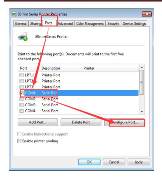
Select available computer COM port, such as "COM1" as the above picture, and then click "Configure Port" to set the detailed parameter.
