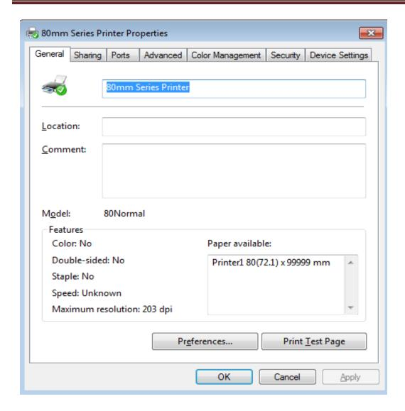
On 80 Printer Properties "General", you could configure the printer communication port, such as Serial port, Parallel port and USB port. You also could set the paper specification, beeper etc.
