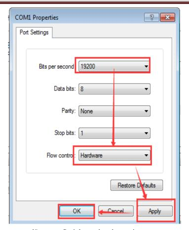
"Bit per second" means Serial port baud rate, it must same as printer setting. For example, if printer baud rate is "19200bsp", then you must select "19200" on "Bit per second", just as above picture. (Factory default baud rate is 9200bps)
